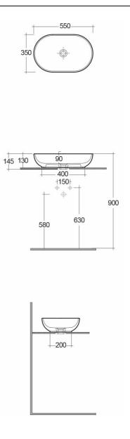
Dimensions: All dimensions in mm tolerance ±5% for below 200mm and ±3% for above 200mm.
